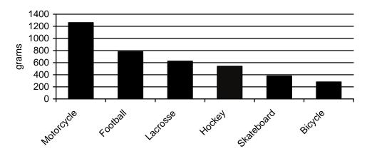
FIGURE 1—Typical weight comparison for several types of helmets.
